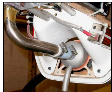
Milled bulkhead around the front of the mini-pipe is also protected from heat with a split silicone tube, that is supplied in the kit.
