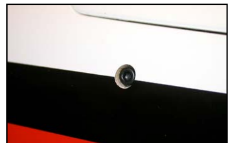
(above) Counterbore the 4 holes for the canopy fixing bolts so that the bolt heads sit against the plywood plates inside the fuselage.
