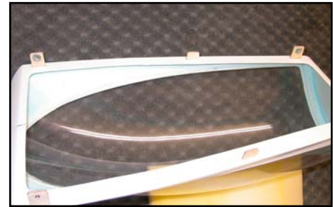
(below) Use masking-tape handles to pull the clear canopy tightly against the canopy frame while gluing it in position.
