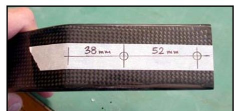
(below) drill 2 x 6.5mm Ø holes for bolting in the Landing Gear.
