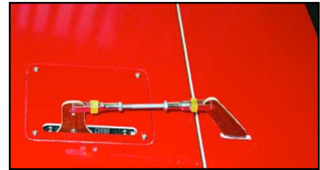
The completed aileron linkage. Note locknuts used at both ends of linkage, and short pieces of tubing used on all quick-links to prevent them opening in flight.
