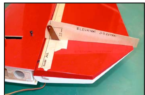
(above) Shows C-ARF servo arm glued and screwed onto standard 25mm diameter servo output arm.
