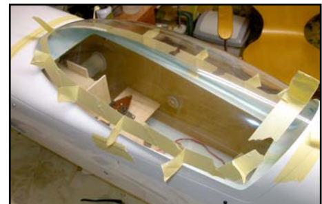
(below) Use masking-tape handles to pull the clear canopy tightly against the canopy frame while gluing it in position.
