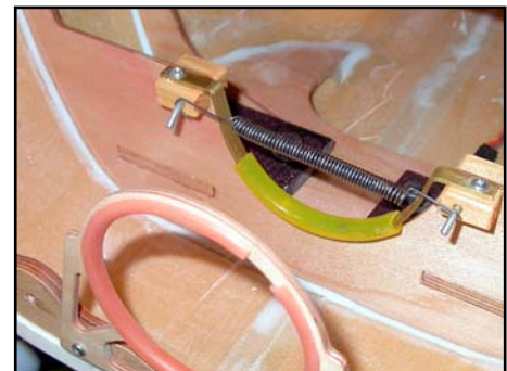
(below) Detail of the mounting strap, protected with a silicone tube, and the spring that goes over the pipe, hooked over 2 steel wires glued into the blocks.
